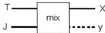
Figure 16.1. Observed signals X (and possibly Y ) are related to target T and jammer J via a mixing matrix. The goal is to derive information about the target T .
