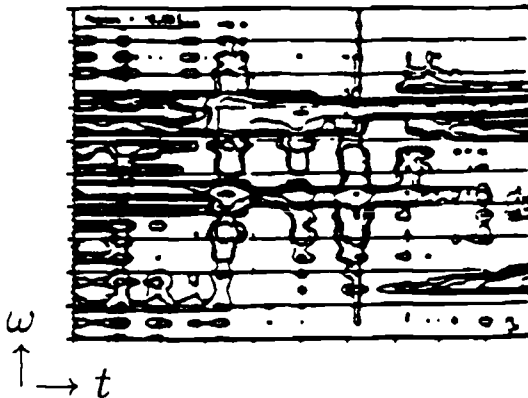
Fig. 5.7 A time-frequency plot of the pressure wave at a particular point in space coming from a model submarine after it was irradiated by a sonar pulse. The first return is the specular reflection (not shown) and the other returns are due to the reradiation of waves induced in the structure by the impeding wave. (From the work of C. Rosenthal and L. Cohen.)
